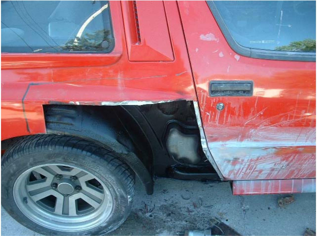
Then I welded in a rust free panel from a donor car and treated the inside as best as I could when done.
