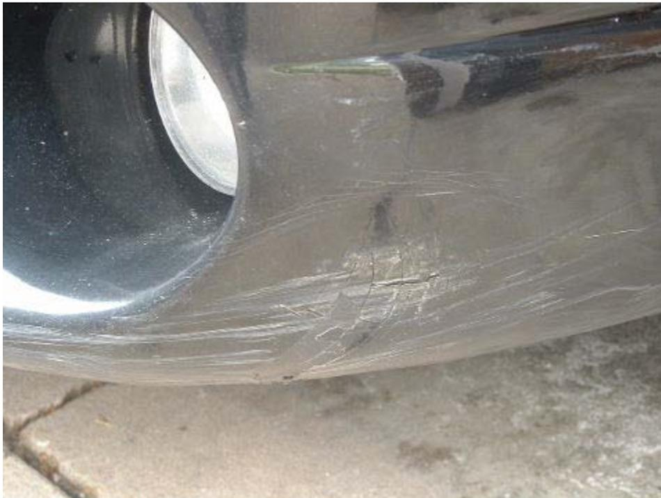
The back was a spot where the factory filler on the bumper was destroyed and chipped out. I used an epoxy type system for bumper repair made by 3M.
