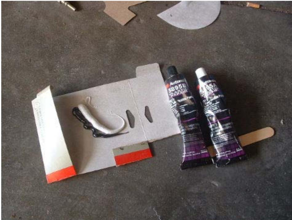
After preliminary sanding to get the paint feather-edged I applied the special two-part bumper filler.
