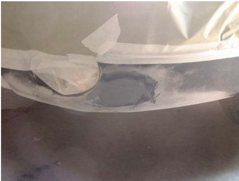
I applied the same stuff to fill in the void of the back bumpers. When fixing cracks, its best to kinda "groove" out the crack before applying the bumper filler.
