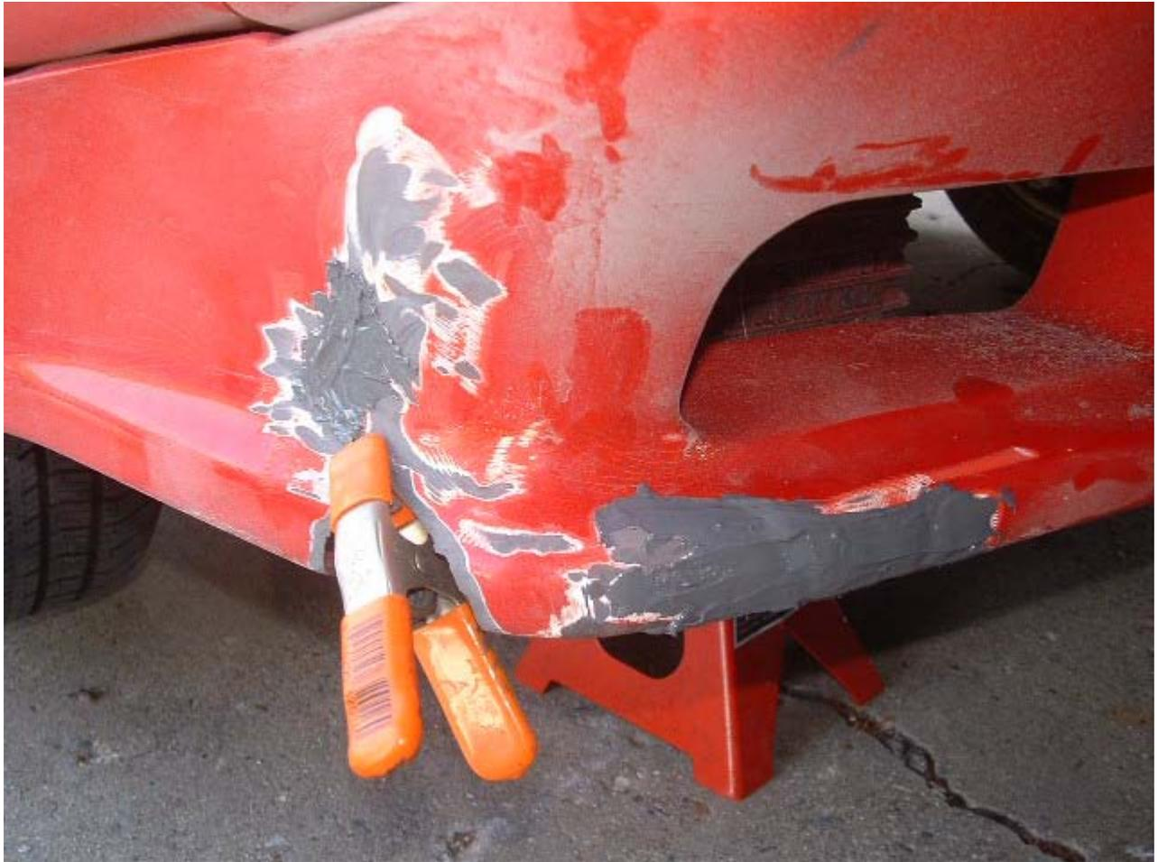
A little fiberglass matting and resin to fill in the big voids- this was then top-coated with the automix and sanded to contour, then primed.
