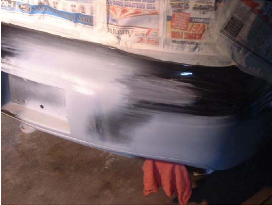
After all is done its time to move to paint. If you are not having it professionally painted, at least paint over the primer as it is porous and will allow water in under the repair.
